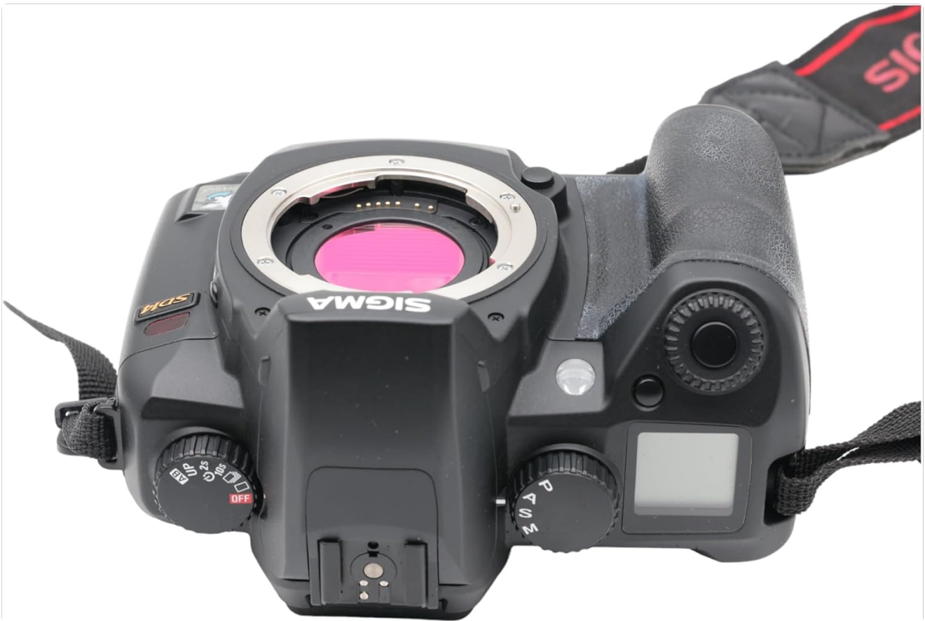
Figure 3.1: Top view of the Sigma SD14, illustrating the lens mount and mode dials.
