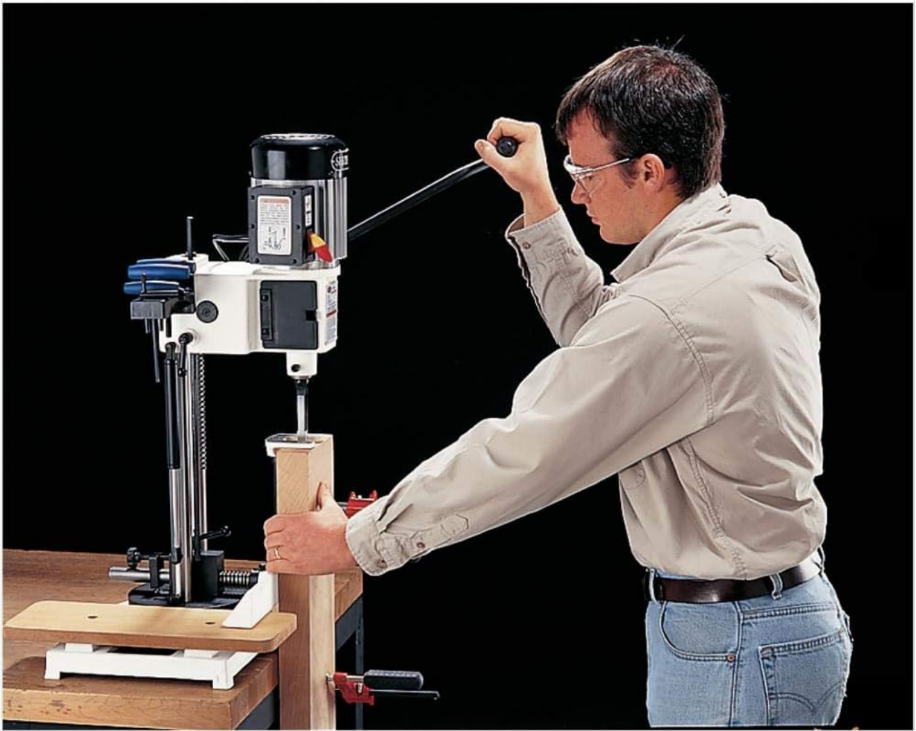
Figure 4: Proper operation of the mortising machine, demonstrating how to apply pressure using the handle.
