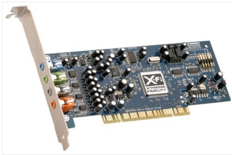
Figure 3: Angled View of Creative Labs SB0790 PCI Sound Card
