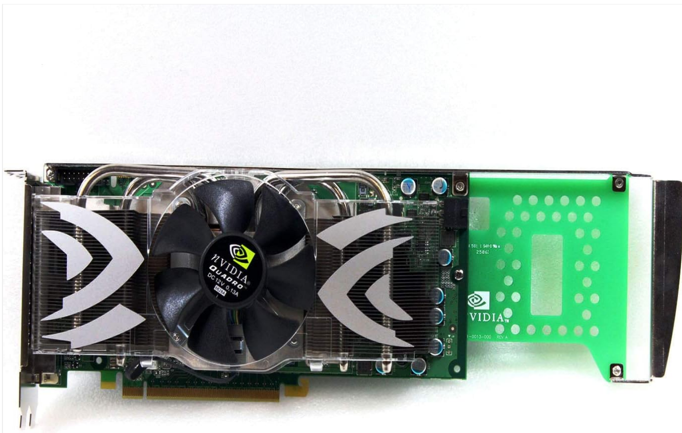
Figure 2: Top-down view of the graphics card, showing the central cooling fan and the heatsink fins beneath the transparent shroud.
