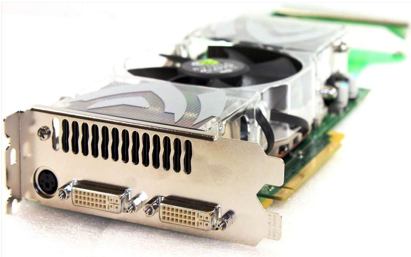
Figure 1: Front view of the Nvidia Quadro FX5500 graphics card, highlighting the dual DVI output ports and the large cooling fan assembly.
