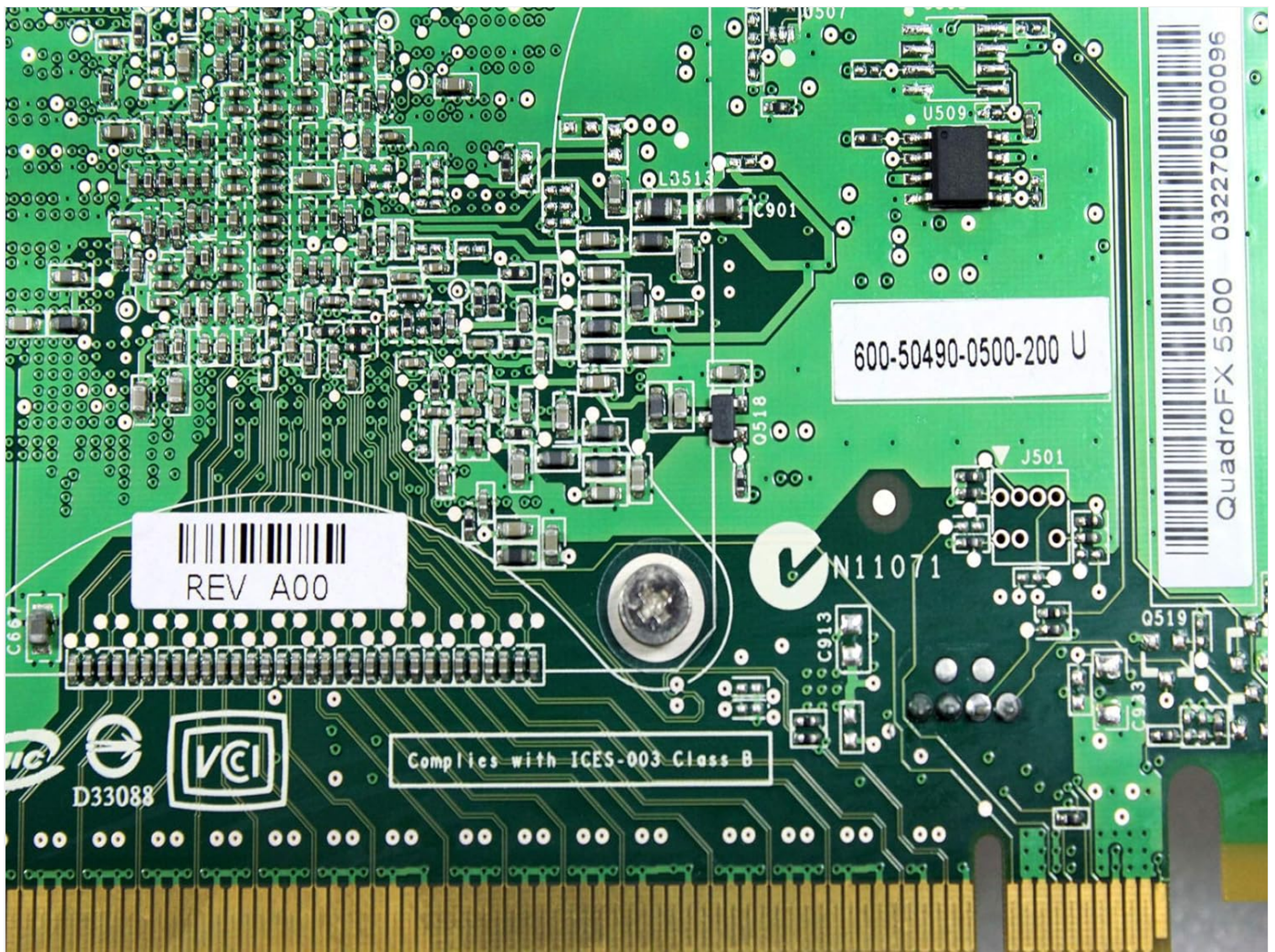
Figure 5: Close-up of the PCB illustrating a revision number (e.g., A00 ) and other circuit details.
