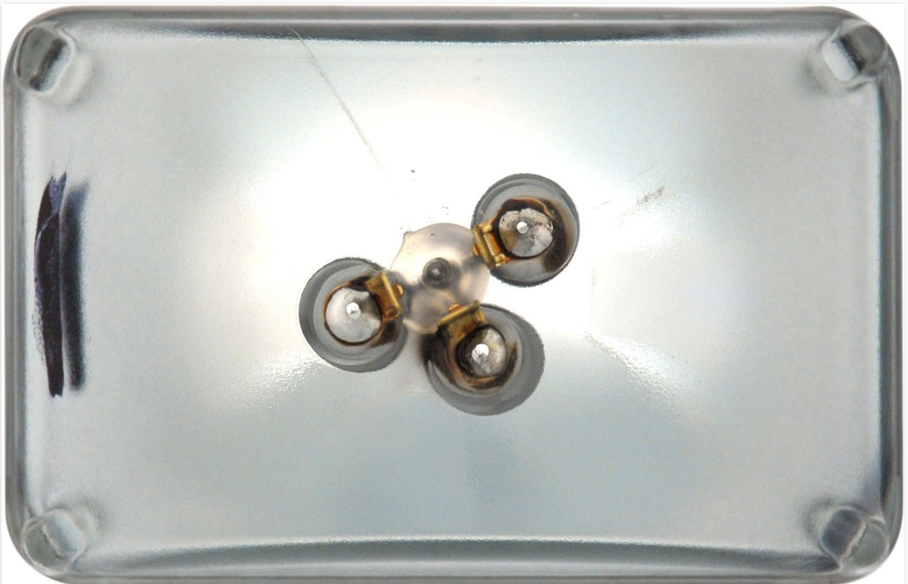
Figure 2: Rear view of the H4656 headlight, illustrating the three electrical terminals for connection.
