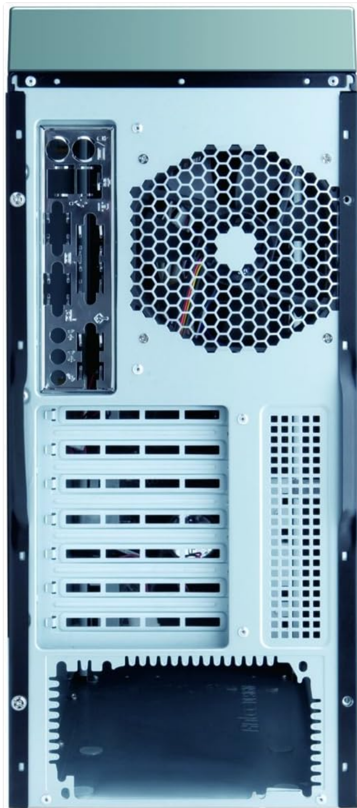
Figure 3.2: Rear panel of the Antec Nine Hundred, highlighting the I/O shield area and expansion slots.
