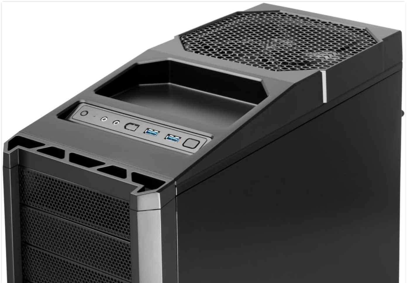
Figure 4.1: Top I/O panel of the Antec Nine Hundred, featuring USB 3.0 ports, audio jacks, and control buttons.
