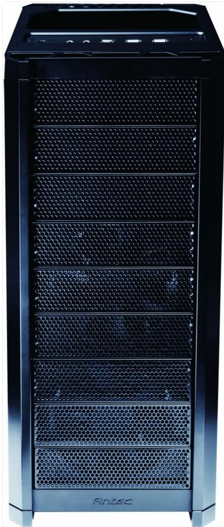
Figure 3.3: Front view of the Antec Nine Hundred, illustrating the accessible drive bays.
