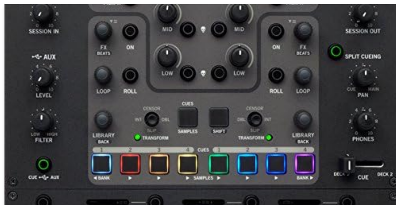
Figure 2: Detailed view of the central control section, highlighting channel controls, effects, and Serato integration buttons.
