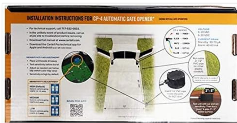
Figure 1: Installation instructions and diagrams from the back of the product box, detailing sensor placement and wiring.
