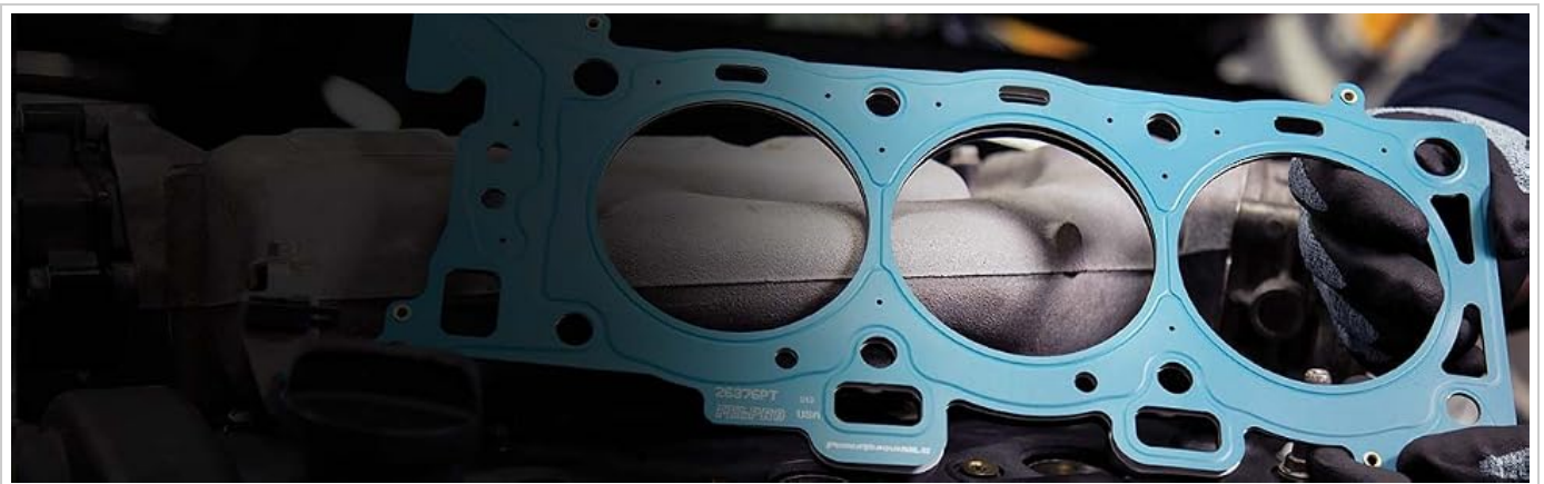
Figure 4.1: Example of a gasket being placed on an engine component. This illustrates the careful handling and positioning required during installation to ensure a proper seal.
