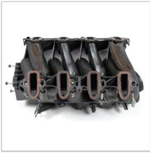
Image: A view of an intake manifold component, showing the surfaces where the gasket will be installed.
