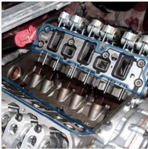
Image: An engine bay with a gasket visibly installed, demonstrating the final placement of the component.
