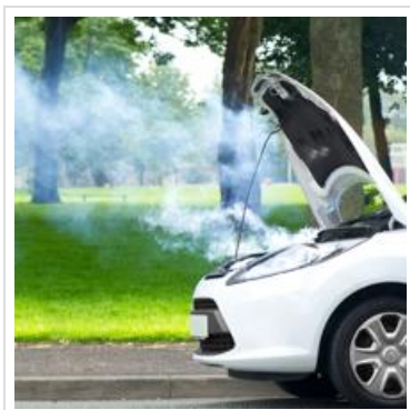
Image 7.1: A vehicle with smoke emanating from the engine bay, a potential sign of a head gasket failure or other engine issue.
