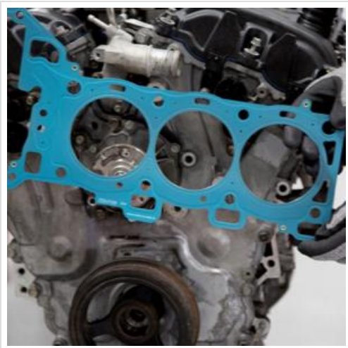
Image 4.2: A technician carefully positioning a head gasket onto an engine block during installation.
