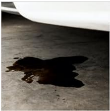
Image: A dark oil stain on a concrete garage floor, indicating a significant engine oil leak.
