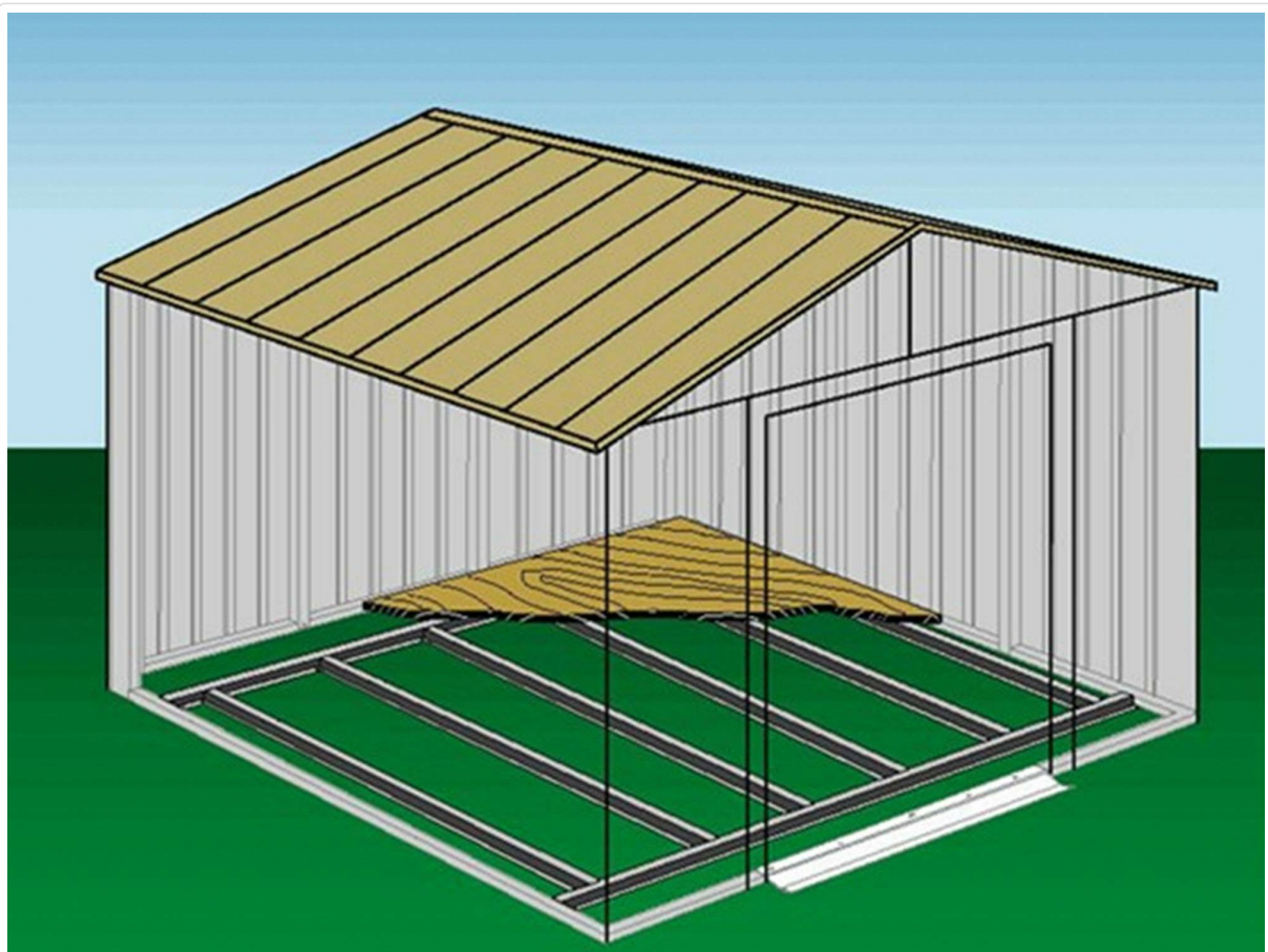
Image: An illustrative diagram showing the complete shed structure with the FB109 Floor Frame Kit and plywood flooring installed at the base.
