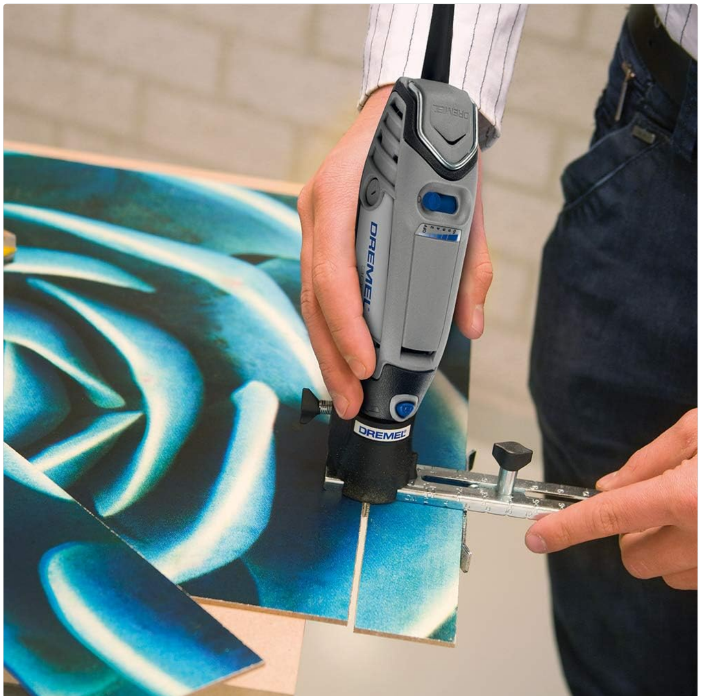
Image: A Dremel rotary tool equipped with the circle cutter attachment actively cutting a circular shape from a patterned material. The user maintains a steady hand while guiding the tool.
