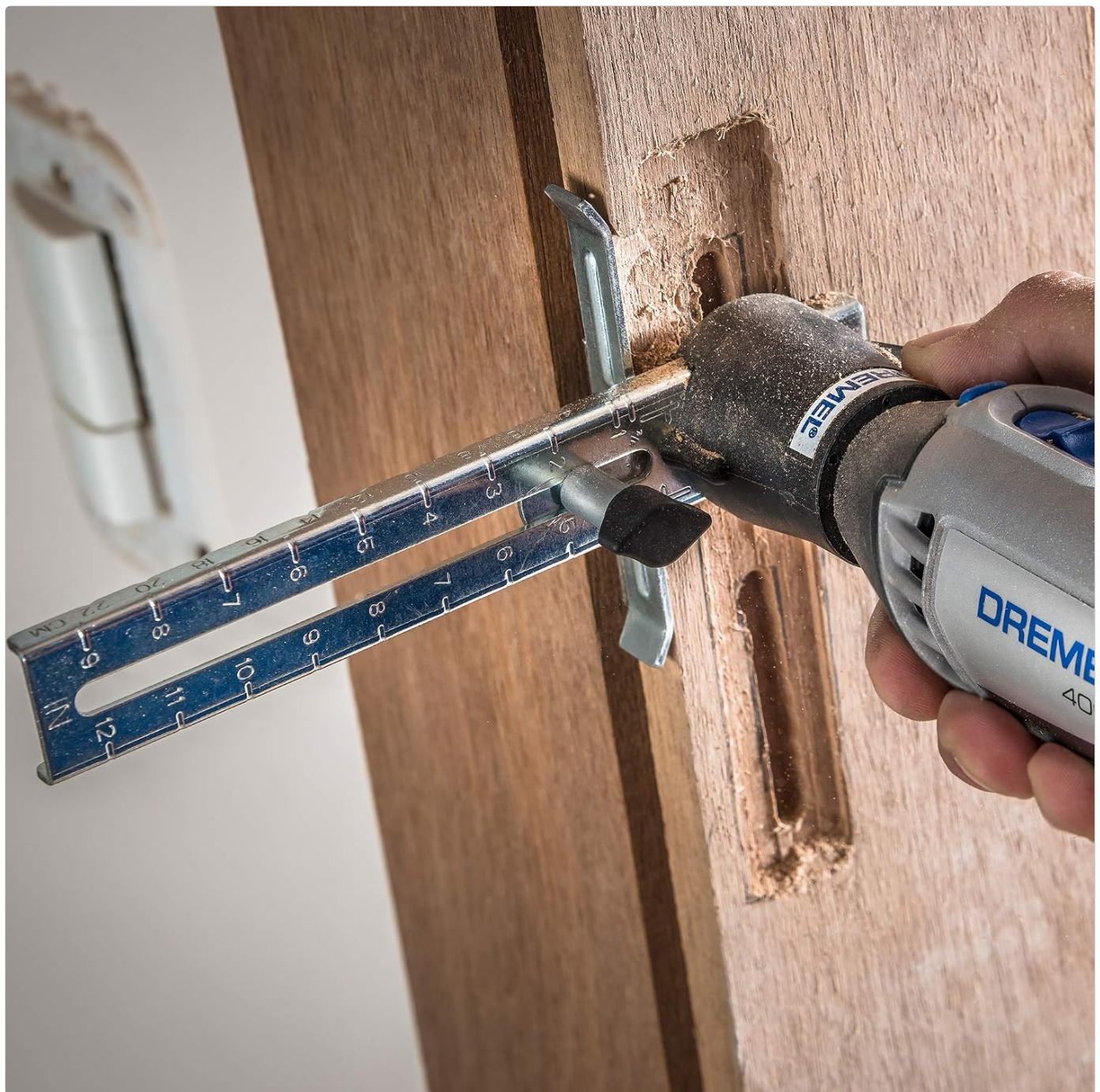
Image: A Dremel rotary tool utilizing the straight edge guide to precisely route a rectangular opening in a wooden door, demonstrating its use for straight-line cuts.
