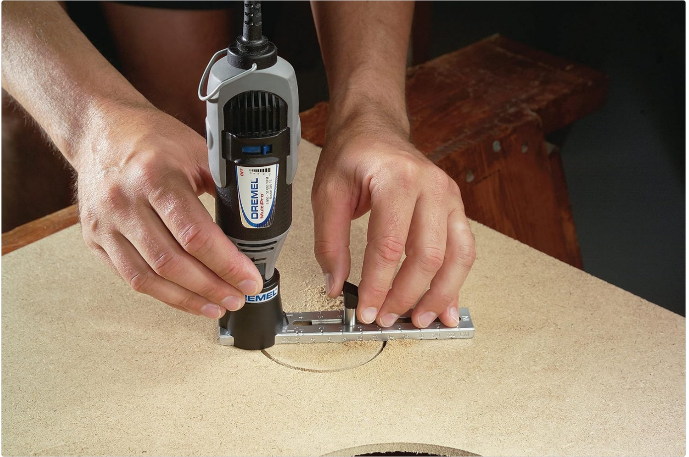
Image: A user adjusting the guide arm of the Dremel 678 attachment to set the desired radius for a circular cut, utilizing the integrated measurement markings.
