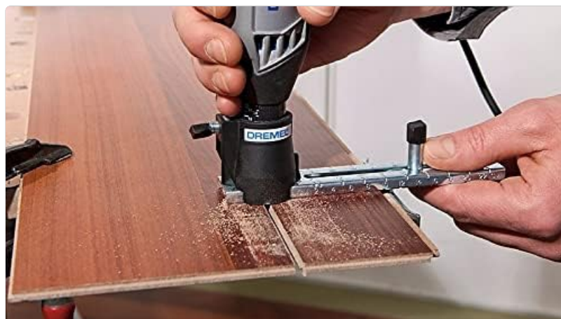
Image: The Dremel 678 attachment configured as a straight edge guide, being used to cut a groove into a wooden floorboard, ensuring a consistent and straight cut.
