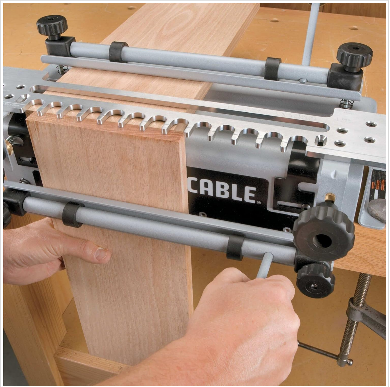
Image: Hands demonstrating the process of securing a wooden workpiece into the jig's clamping mechanism.
