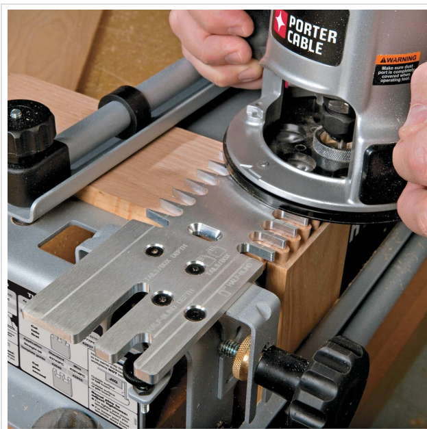
Image: A close-up of the router creating box joints, demonstrating the jig's versatility.
