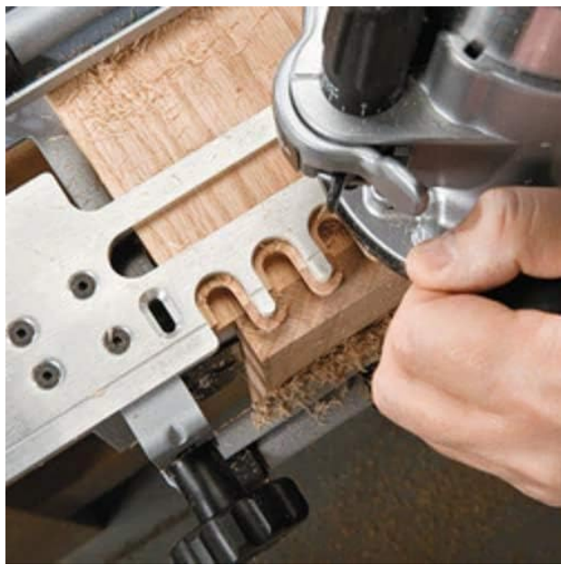
Image: A router in action, cutting half-blind dovetails into a wooden piece using the jig.
