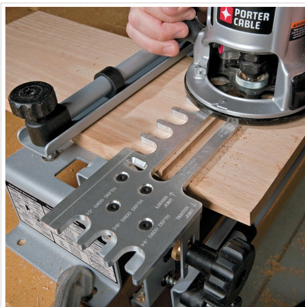
Image: The router precisely cutting through dovetails, guided by the jig's template.
