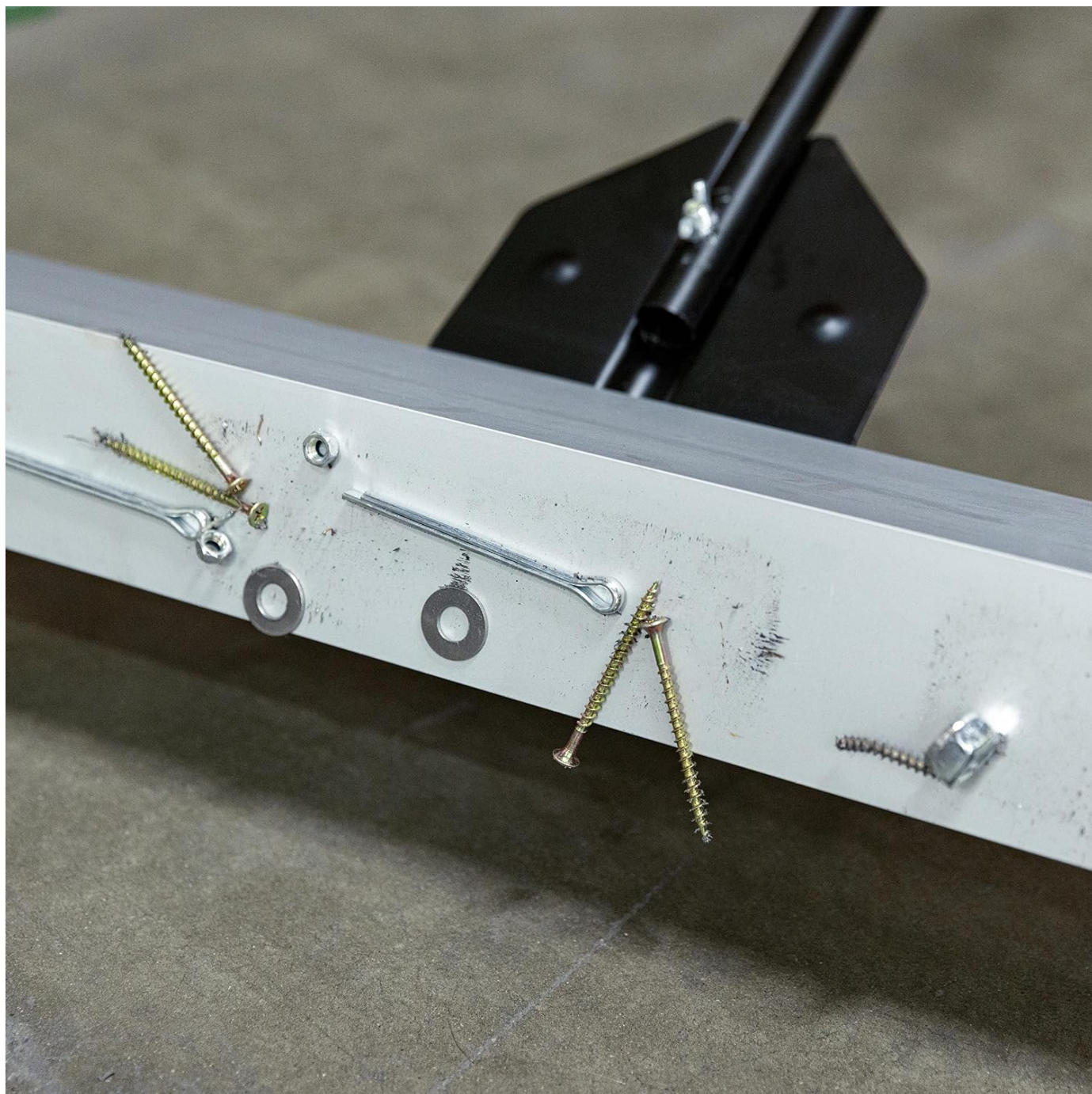
Figure 7: Collected metal debris adhering to the sweeper's magnetic surface.
