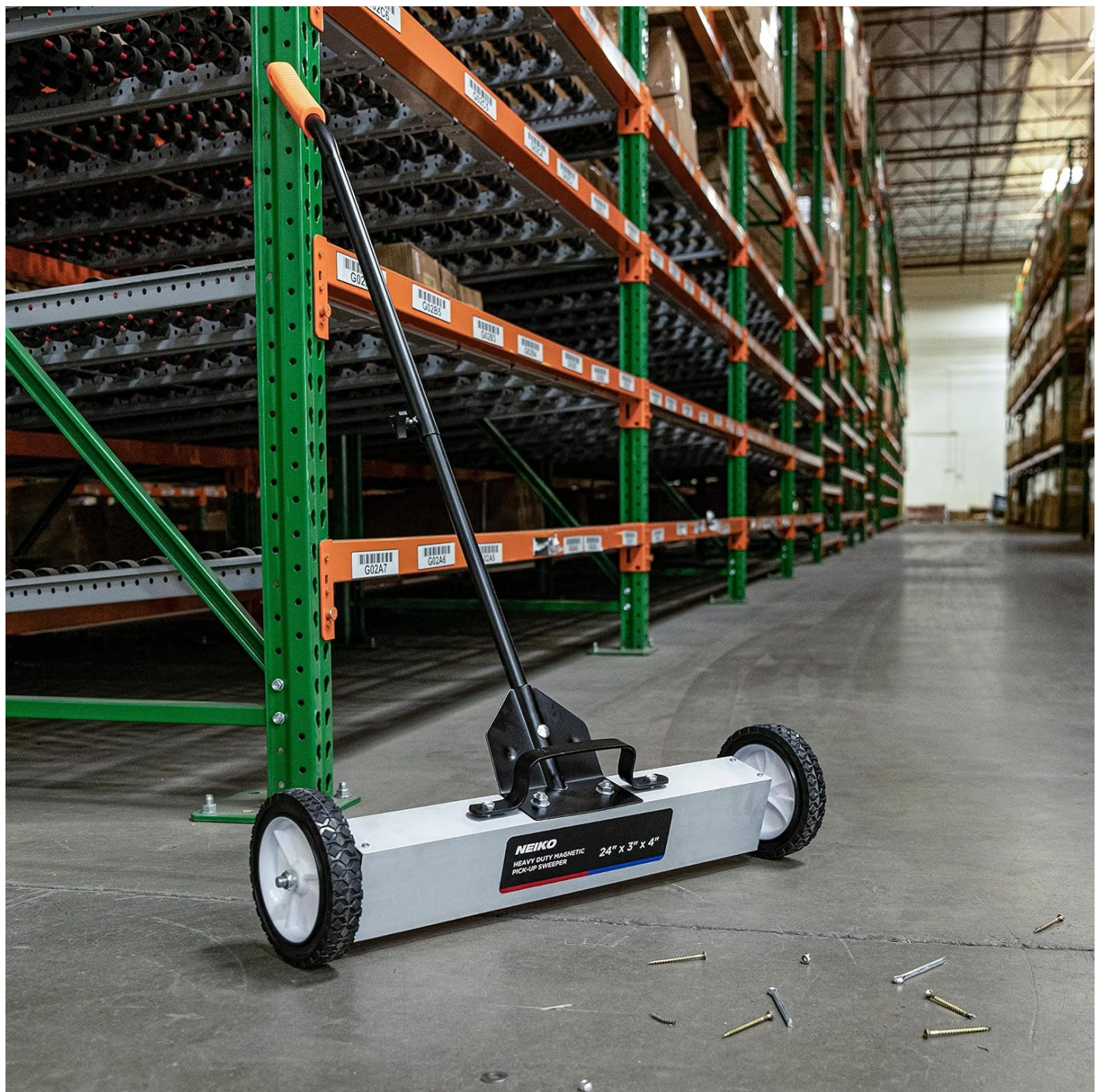
Figure 4: Magnetic sweeper in operation on a shop floor.
