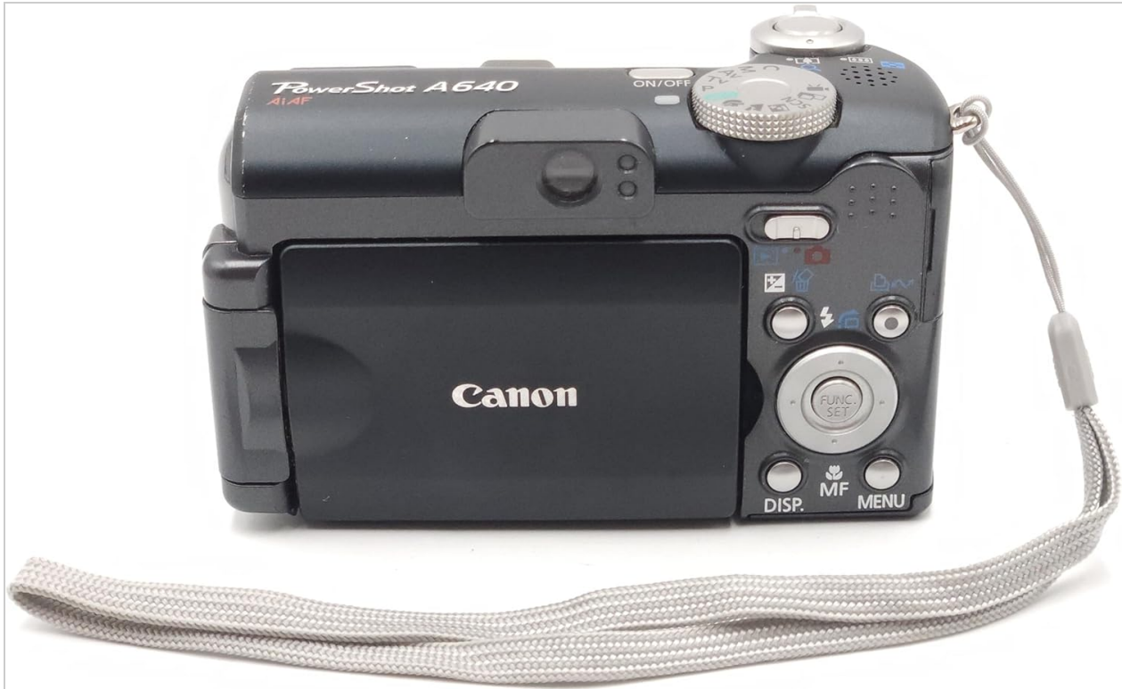
Image 4: Rear view of the Canon PowerShot A640, showing the vari-angle LCD and navigation controls.
