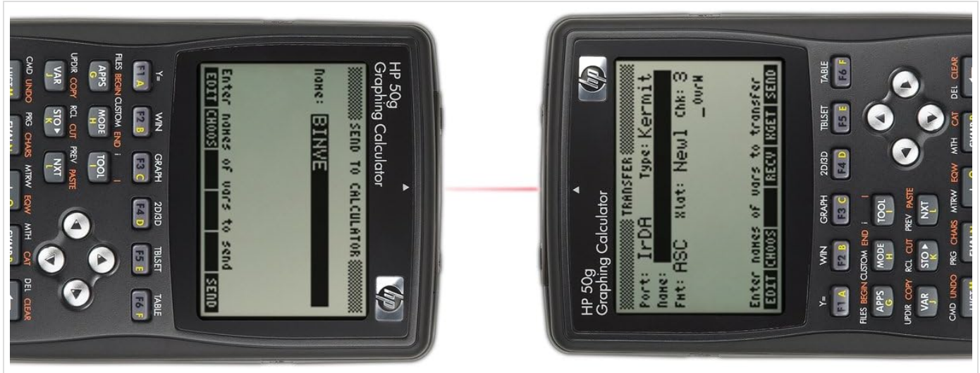
Figure 2.2: Infrared data transfer between two HP 50g calculators.
