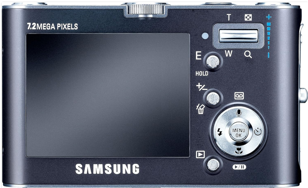
Figure 2: Rear view of the Samsung NV3 Digital Camera, showing the LCD screen and various control buttons for navigation and settings.
