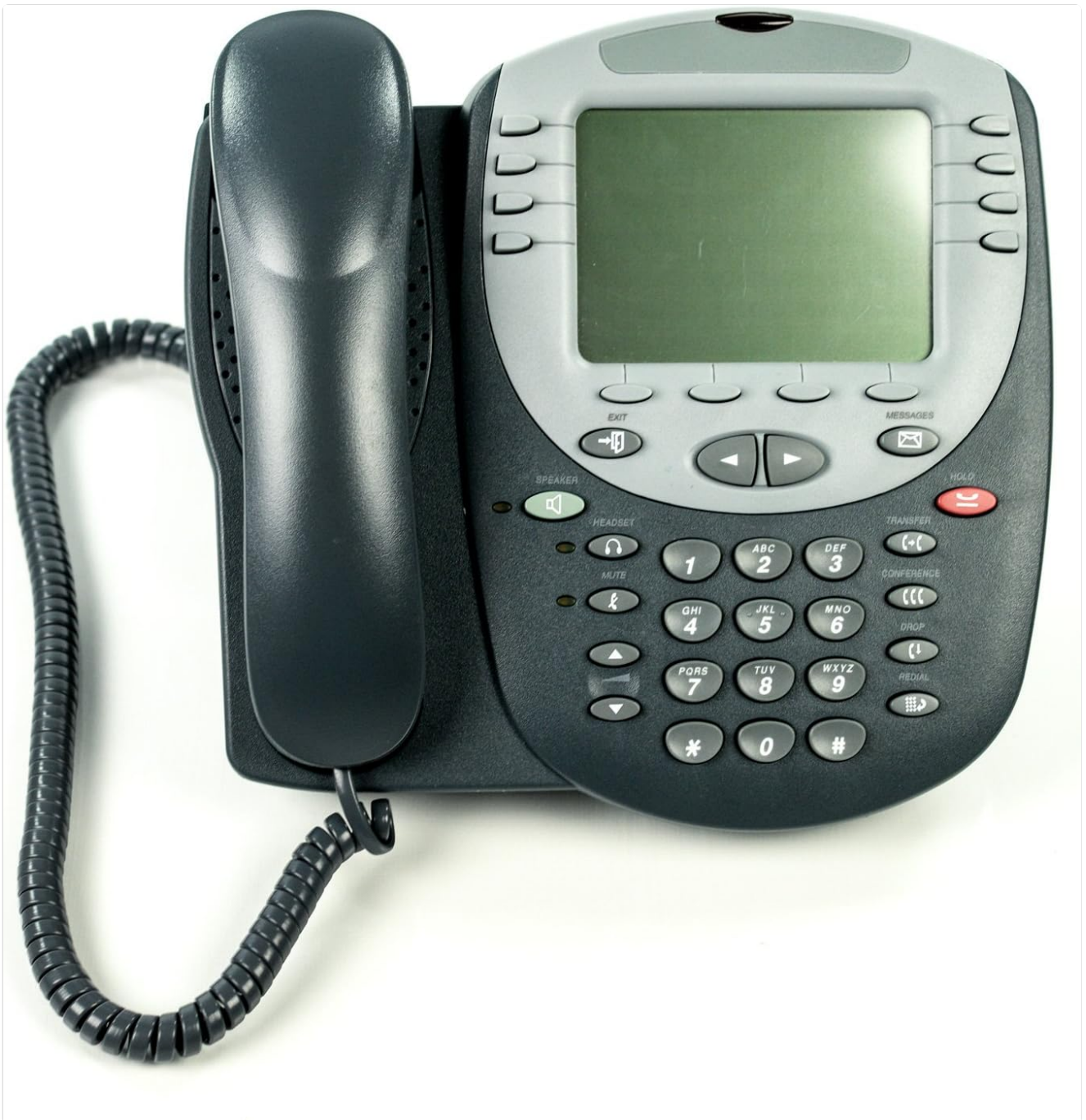
Figure 4.2: Top-down view of the Avaya 2420 Digital Telephone, highlighting the display, navigation buttons, and keypad for various functions.
