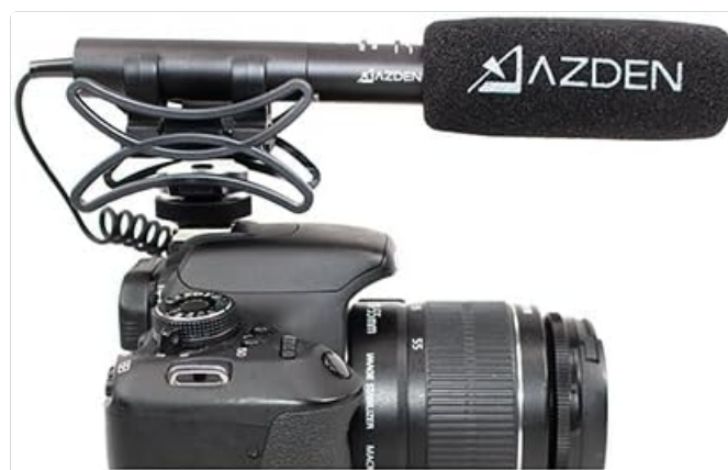
Figure 2: Azden SMX-10 microphone with its foam windscreen attached to a camera, viewed from the side.
