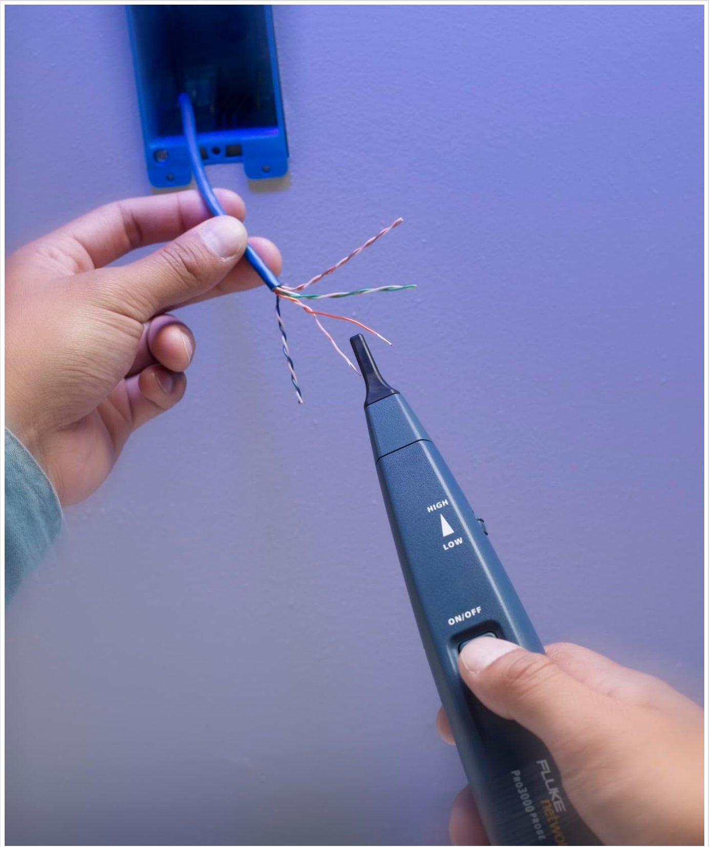
Figure 6.1: The Pro3000 Probe being used to identify individual wires from a bundle connected to a wall jack. The user holds the probe tip near the exposed wires to detect the tone.
