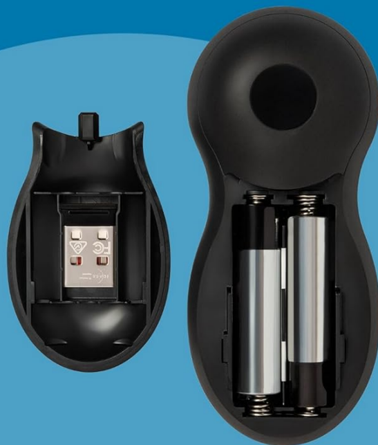
Image: The internal storage compartment of the presenter, showing the space for the USB receiver and two AAA batteries.
