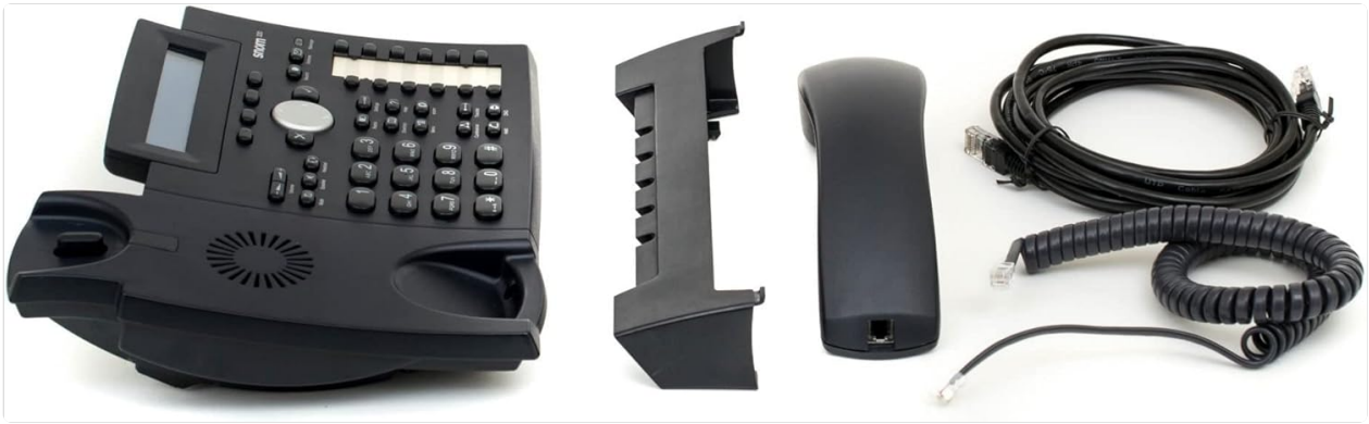
Figure 3.1: Components included with the Snom 320 IP Phone, showing the phone unit, handset, handset cord, Ethernet cable, and phone stand.
