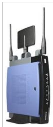
Figure 1: Front view of the Linksys WRT300N Wireless-N Broadband Router, showcasing its compact design with two external antennas and indicator lights.
