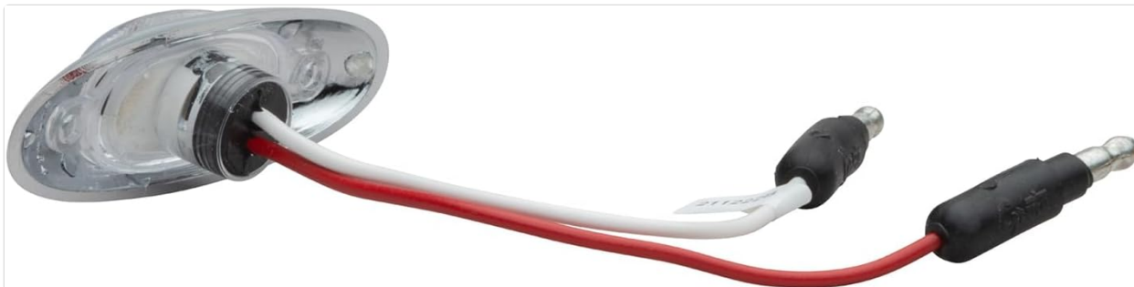
Image: Rear view of the Grote 47982 MicroNova LED Clearance Marker Light, illustrating the red and white wiring for power and ground connections.
