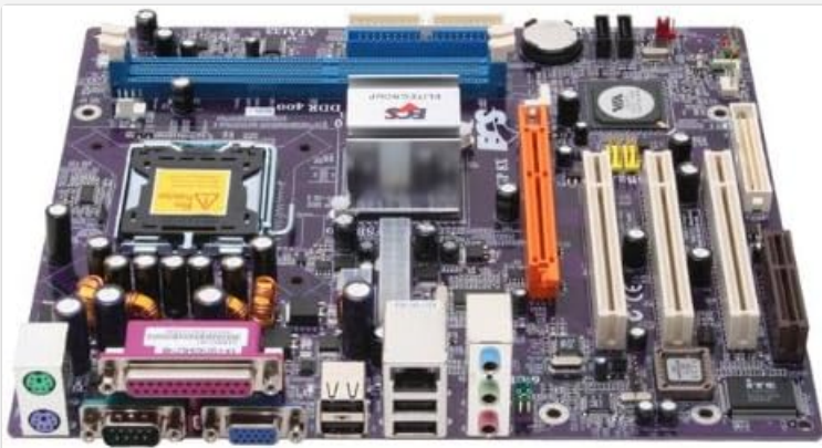
Figure 1: ECS P4M800-M7 Motherboard Layout. This image displays the main components of the motherboard, including the CPU socket (LGA 775), two DDR RAM slots, PCI and AGP expansion slots, and various I/O ports.
