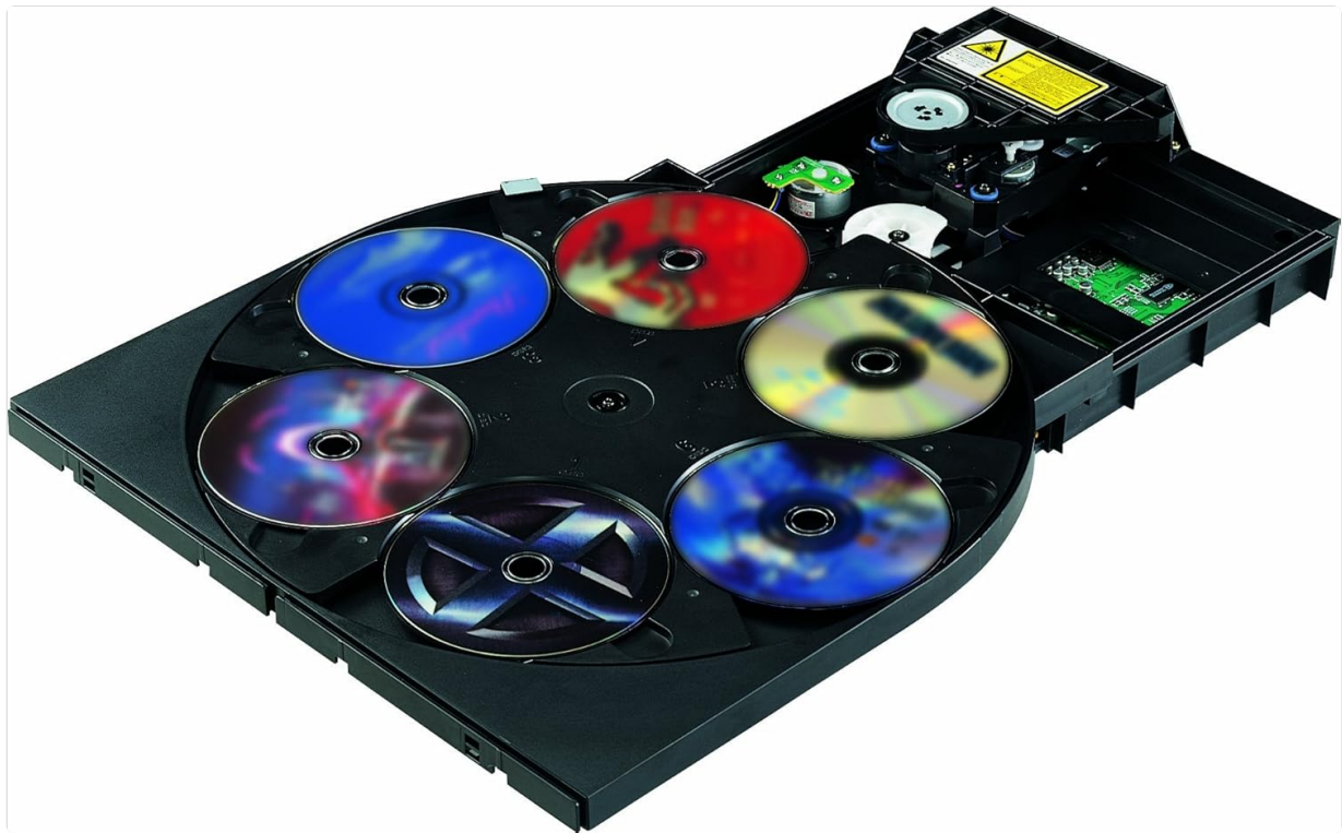
Figure 2: Onkyo DX-C390 6-Disc Carousel Mechanism. This image shows the internal carousel mechanism of the CD changer with multiple discs loaded, illustrating its multi-disc capability.
