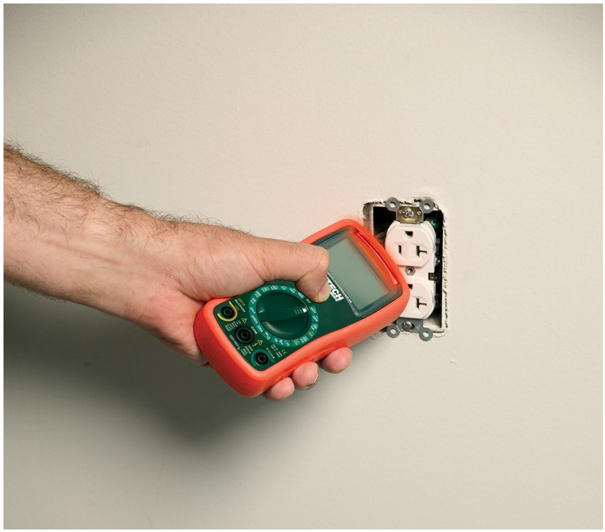
Image: A hand holding the Extech EX310 Multimeter near an electrical wall outlet, demonstrating the use of the Non-Contact Voltage (NCV) detection feature to identify live circuits.
