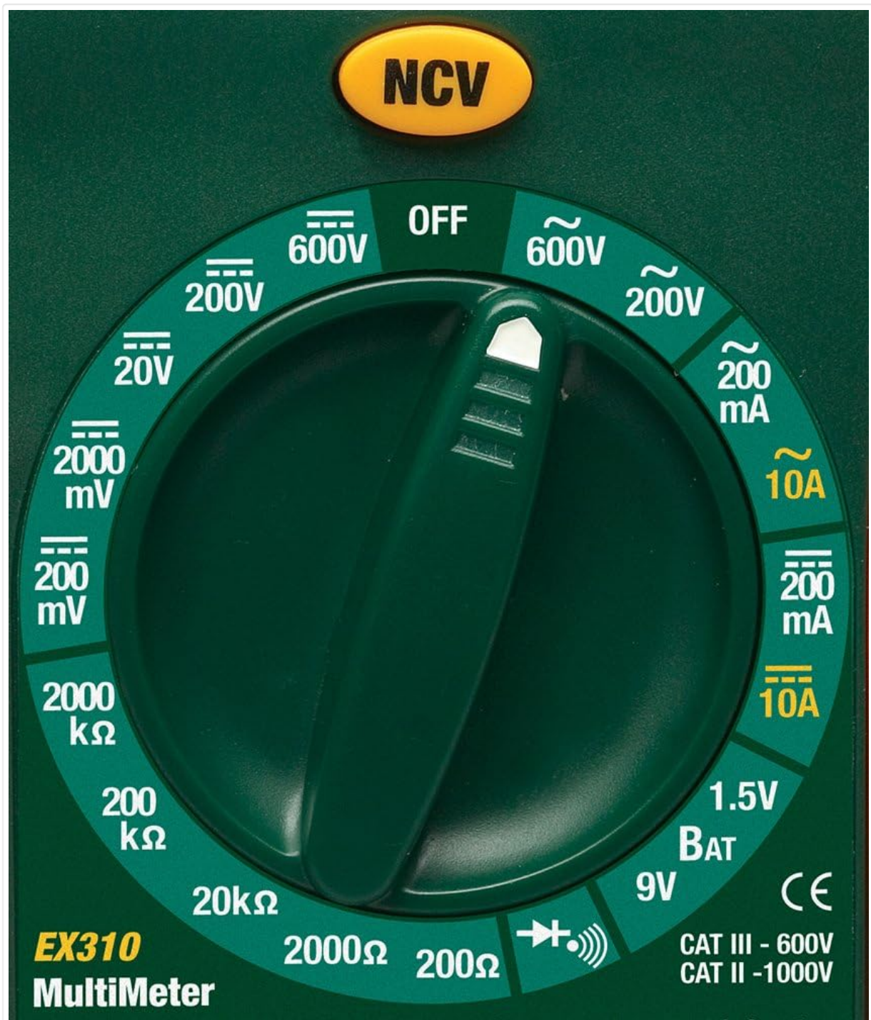
Image: Close-up of the Extech EX310's function dial, illustrating the various measurement ranges and functions such as voltage, current, resistance, diode, continuity, and battery test.
