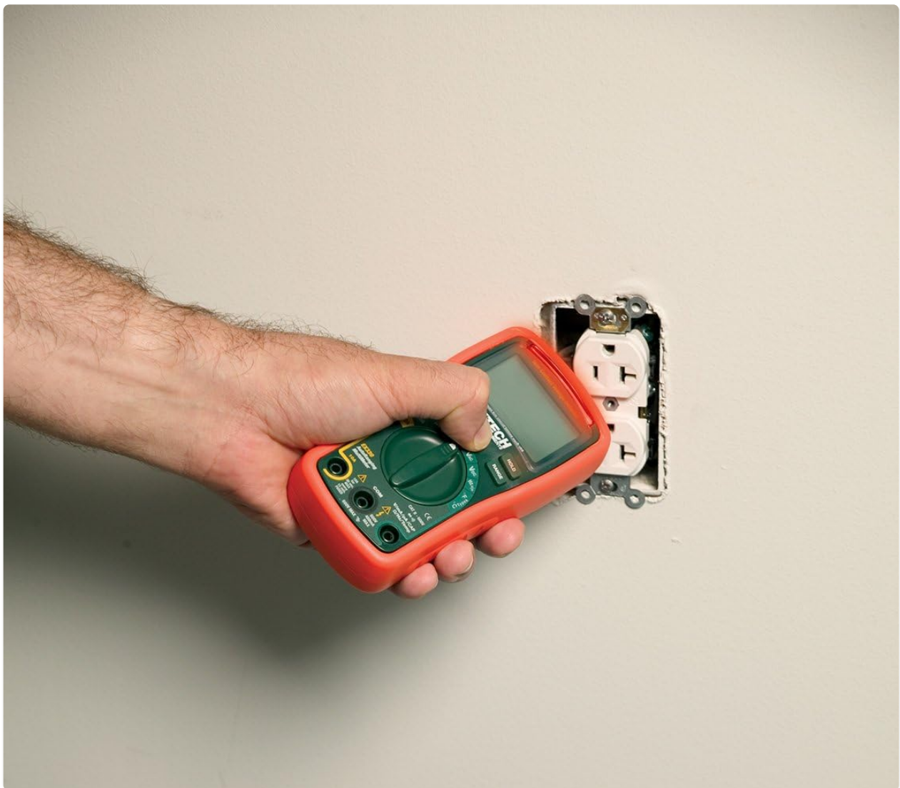
Figure 3.1: Using the NCV feature to detect live AC voltage.
