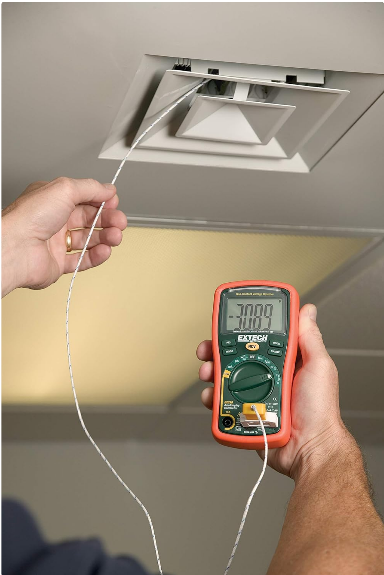
Figure 3.3: Measuring temperature using the Type K probe.
