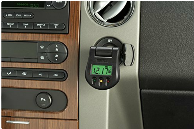
Figure 4.1: Innova 3721 displaying voltage in a vehicle.
