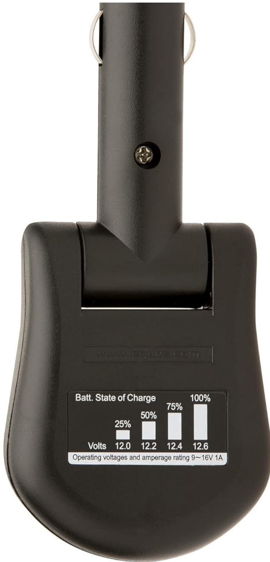
Figure 4.3: Battery State of Charge table on the device.
