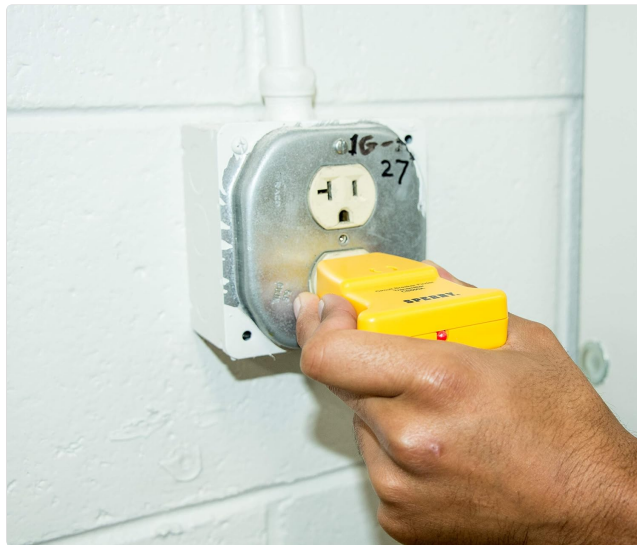
Image: The transmitter unit being plugged into a standard electrical wall outlet.
