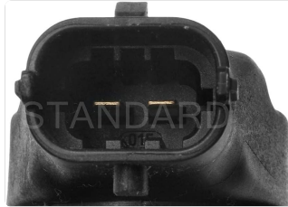
Figure 2.3: Electrical connector for signal input to the injector.
