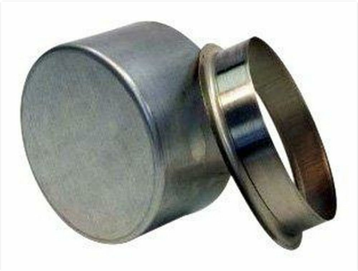
Image 1.1: The SKF Speedi Sleeve and its installation tool. The sleeve is a thin-walled stainless steel component designed to cover worn shaft surfaces.
