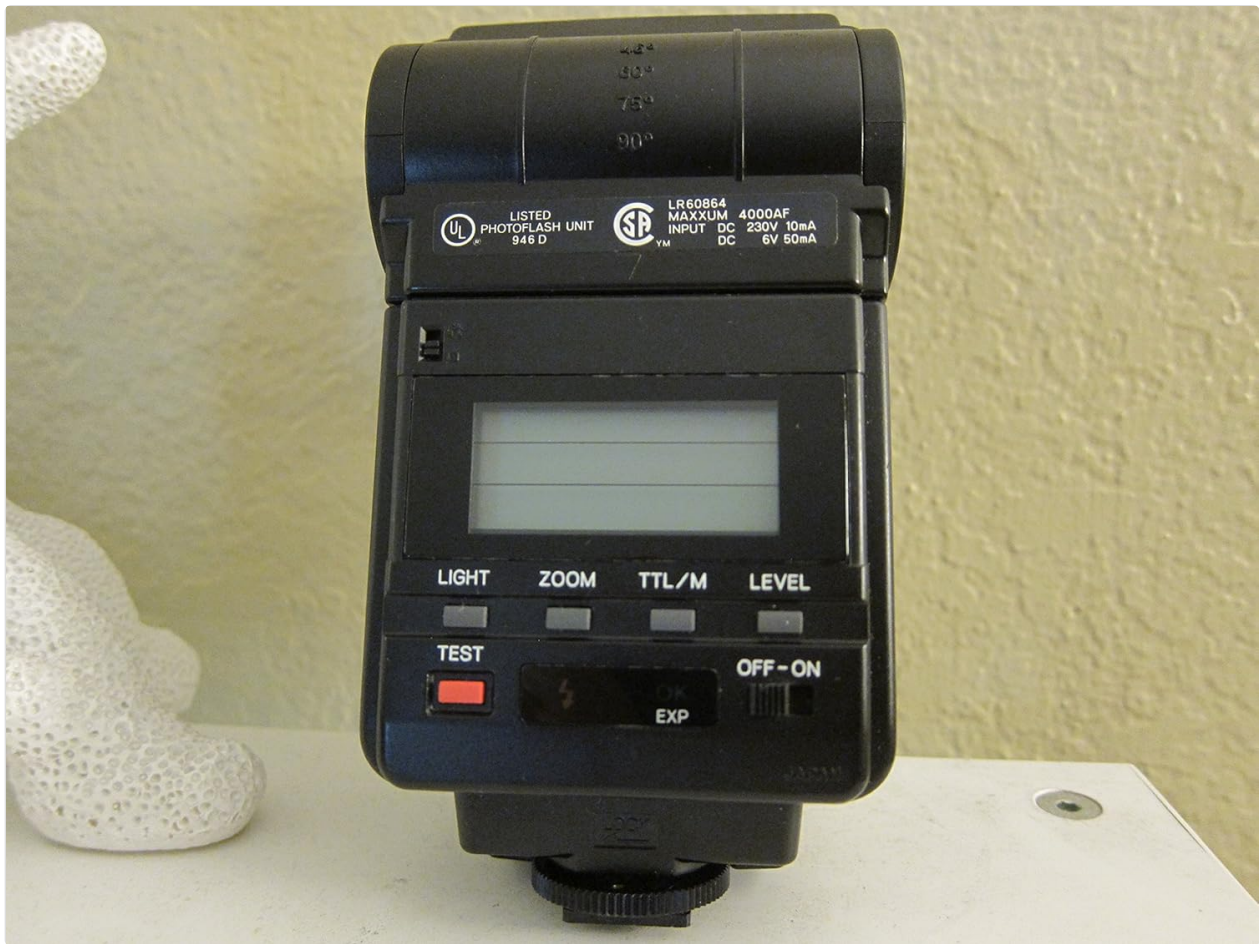
Image: Rear view of the Minolta 4000AF flash unit, showing the control panel. Buttons for LIGHT, ZOOM, TTL/M, LEVEL, and TEST are visible, along with the OFF-ON switch and an LCD display. This panel allows users to adjust flash settings and modes.
