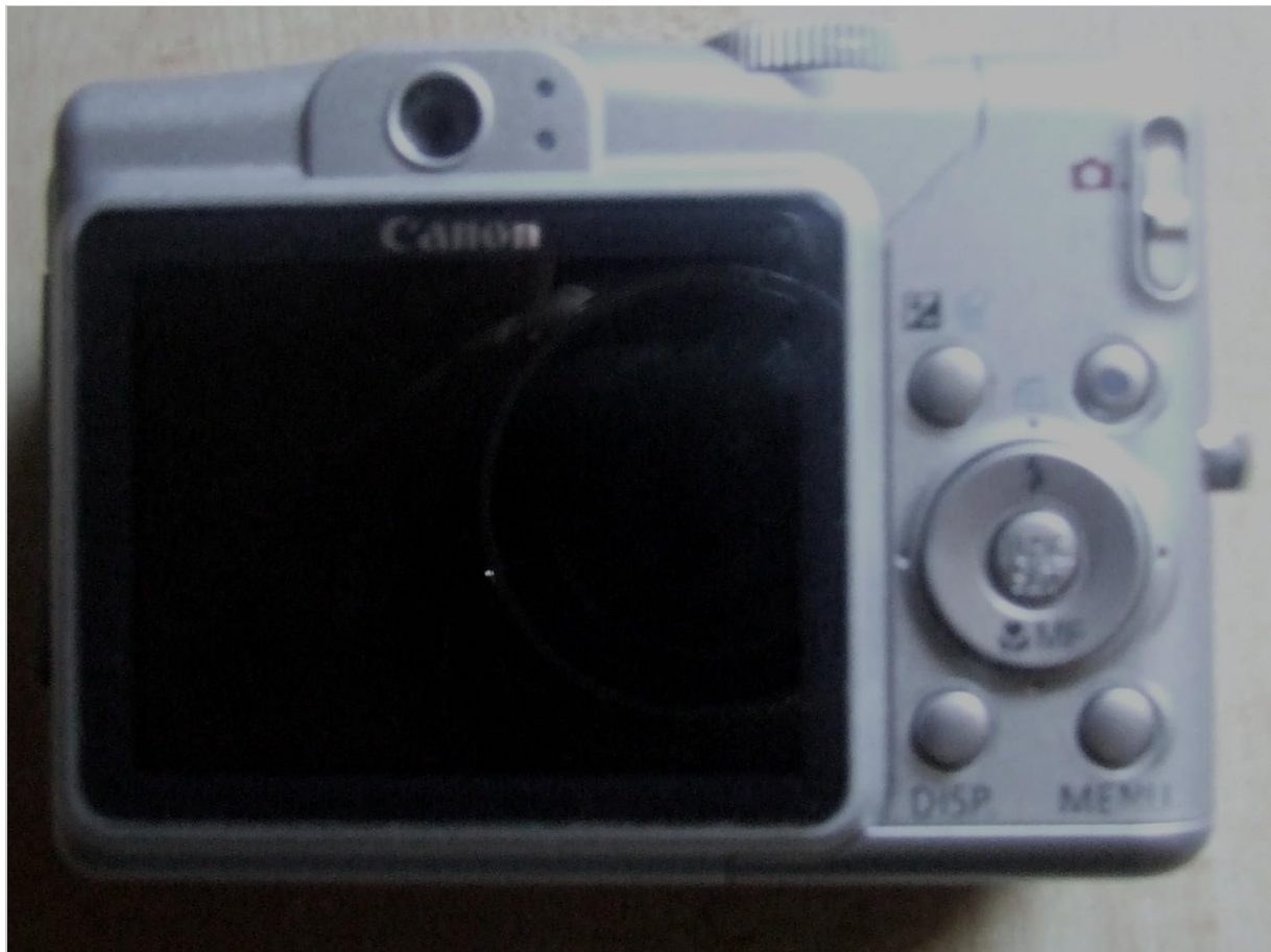
Figure 3: Back view of the Canon PowerShot A700, displaying the 2.5-inch LCD screen and navigation buttons. This image illustrates the user interface for reviewing photos and adjusting settings.
