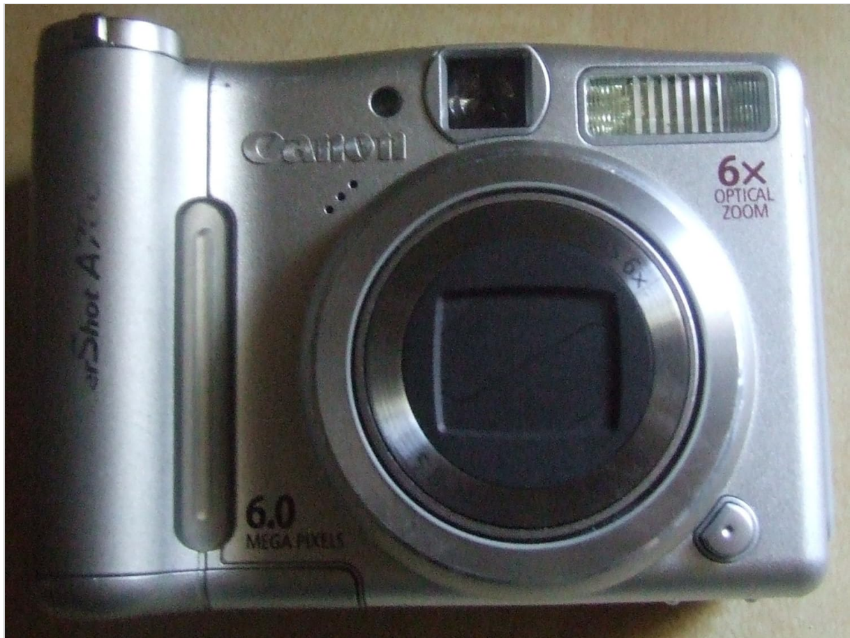
Figure 1: Front view of the Canon PowerShot A700 camera. This image shows the lens, flash, and viewfinder on the front of the camera.
