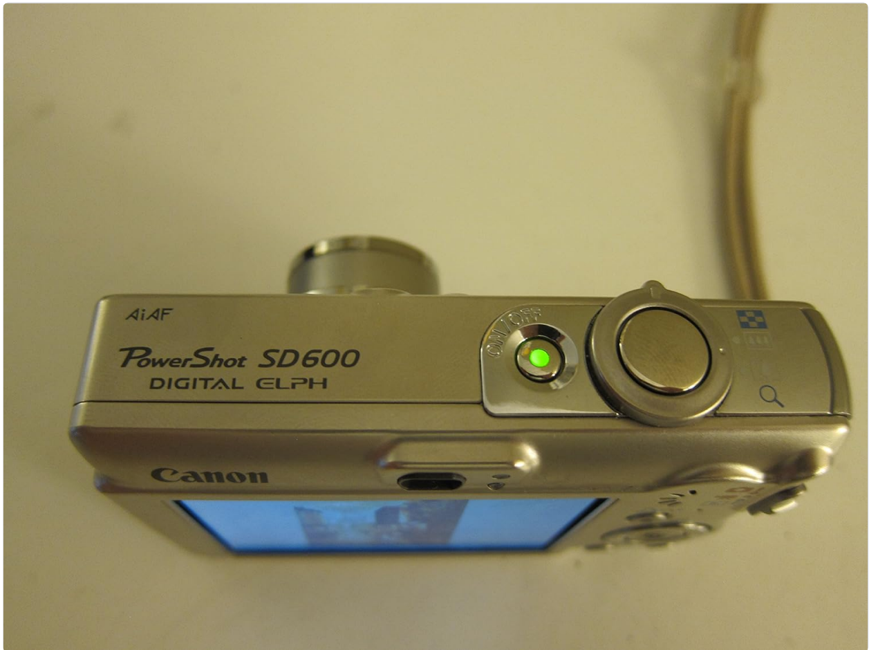
Figure 3.1.1: Top view of the camera, highlighting the ON/OFF button and the shutter button with zoom control.
