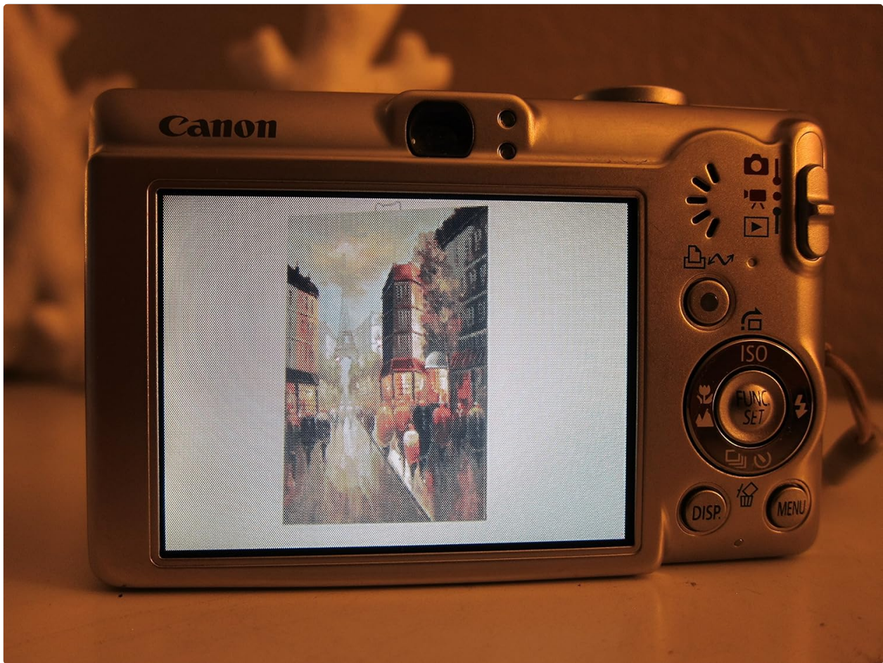
Figure 3.3.1: Rear view of the camera, showing the LCD screen displaying a sample image and the surrounding control buttons for navigation and settings.
