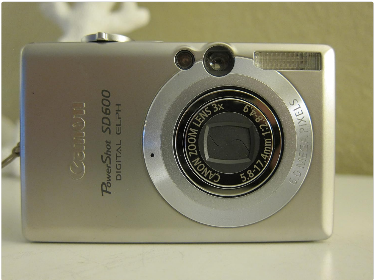
Figure 3.2.1: Front view of the Canon PowerShot SD600, showing the lens, flash, and viewfinder.
