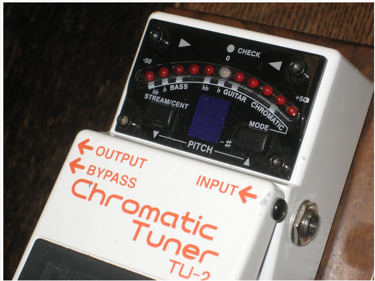
Figure 3.1: Close-up of the TU-2 display. This image shows the 7-segment LED for note names, the 11-point LED indicators for tuning accuracy, and the MODE and PITCH buttons.
