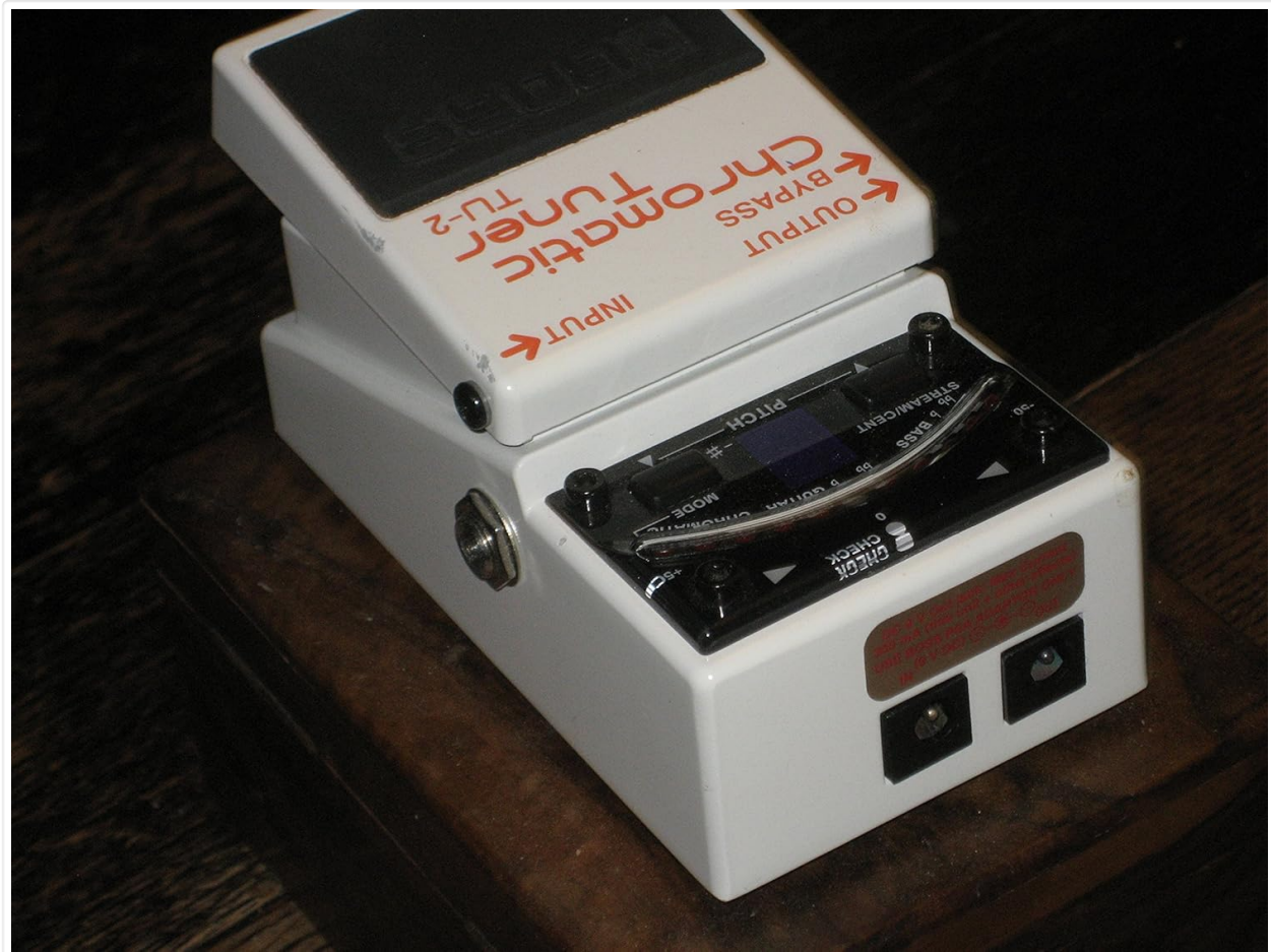
Figure 2.2: Side view of the TU-2 pedal. This image highlights the 1/4-inch input and output jacks for instrument and amplifier connections.
