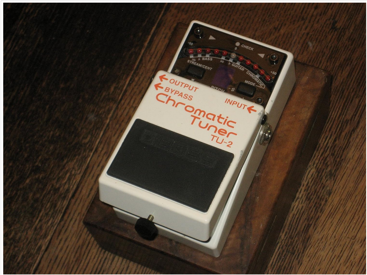
Figure 1.1: The BOSS TU-2 Chromatic Tuner Pedal. This image displays the overall design of the pedal, including the footswitch and the tuning display area.
