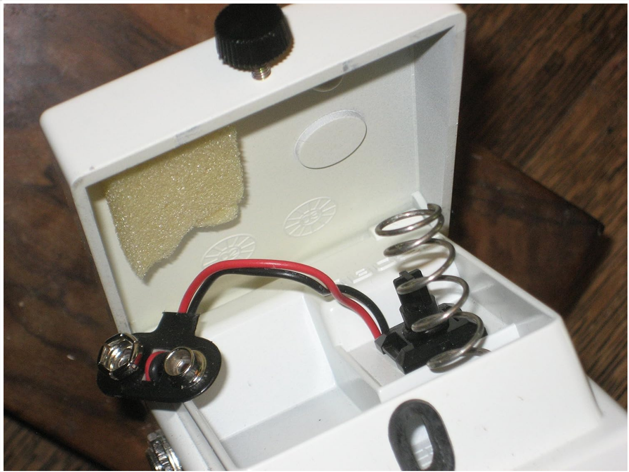
Figure 2.1: Open battery compartment of the TU-2 pedal. This view shows the internal battery connector and space for a 9V battery.
