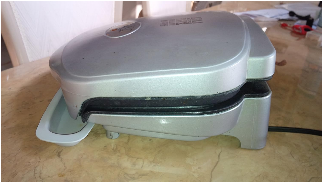
Figure 2: Side view of the George Foreman GR30 Grilling Machine, showing the integrated drip tray positioned to collect fat and grease.
