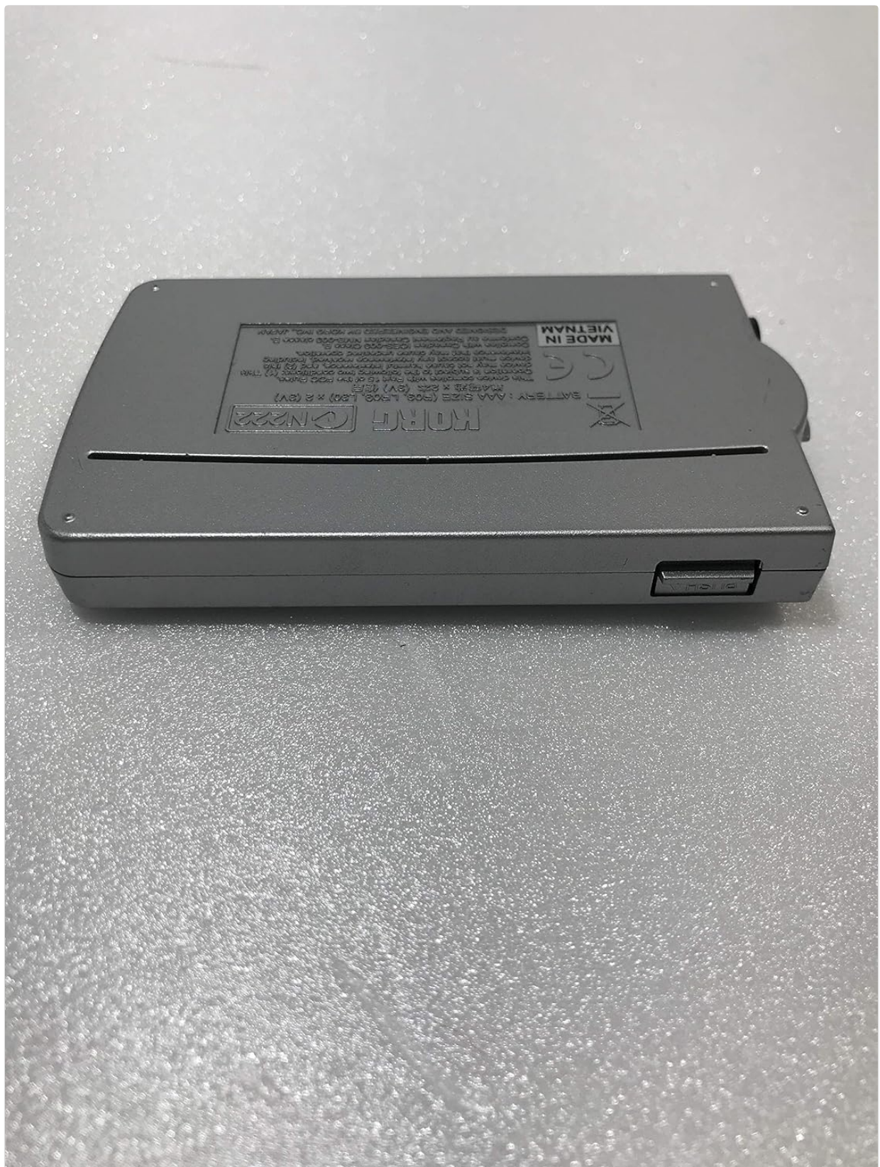
Figure 2: Back view of the Korg GA30 tuner, illustrating the battery compartment and kickstand.
