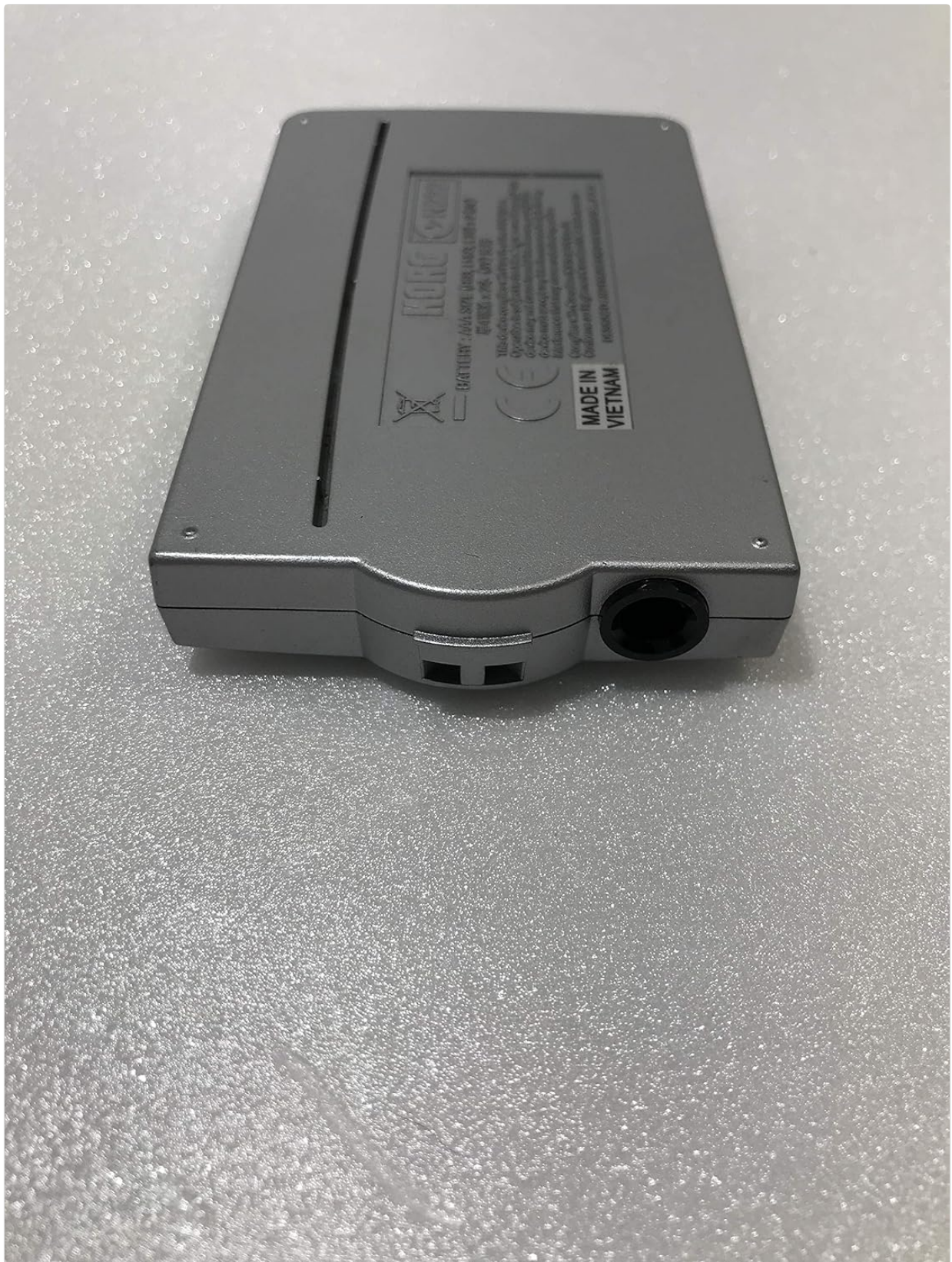
Figure 3: Side view of the Korg GA30 tuner, highlighting the 1/4-inch input jack for direct instrument connection.
