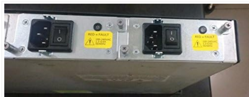
Figure 4.2: Rear view of the controller, highlighting the dual power input modules with power switches and fault indicators.
