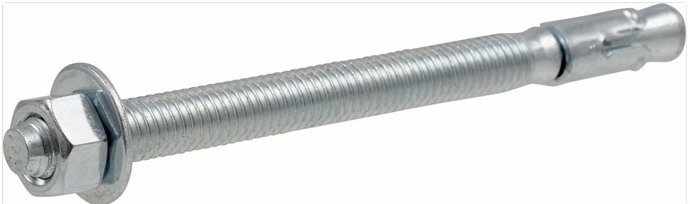
Image: A complete Hillman 3/8 x 5-inch Wedge Anchor, showing the threaded bolt, expansion clip, hex nut, and flat washer.
