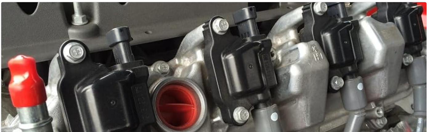
Image: An engine bay illustrating the typical location of ignition coils and spark plugs, which need to be accessed for installation.
