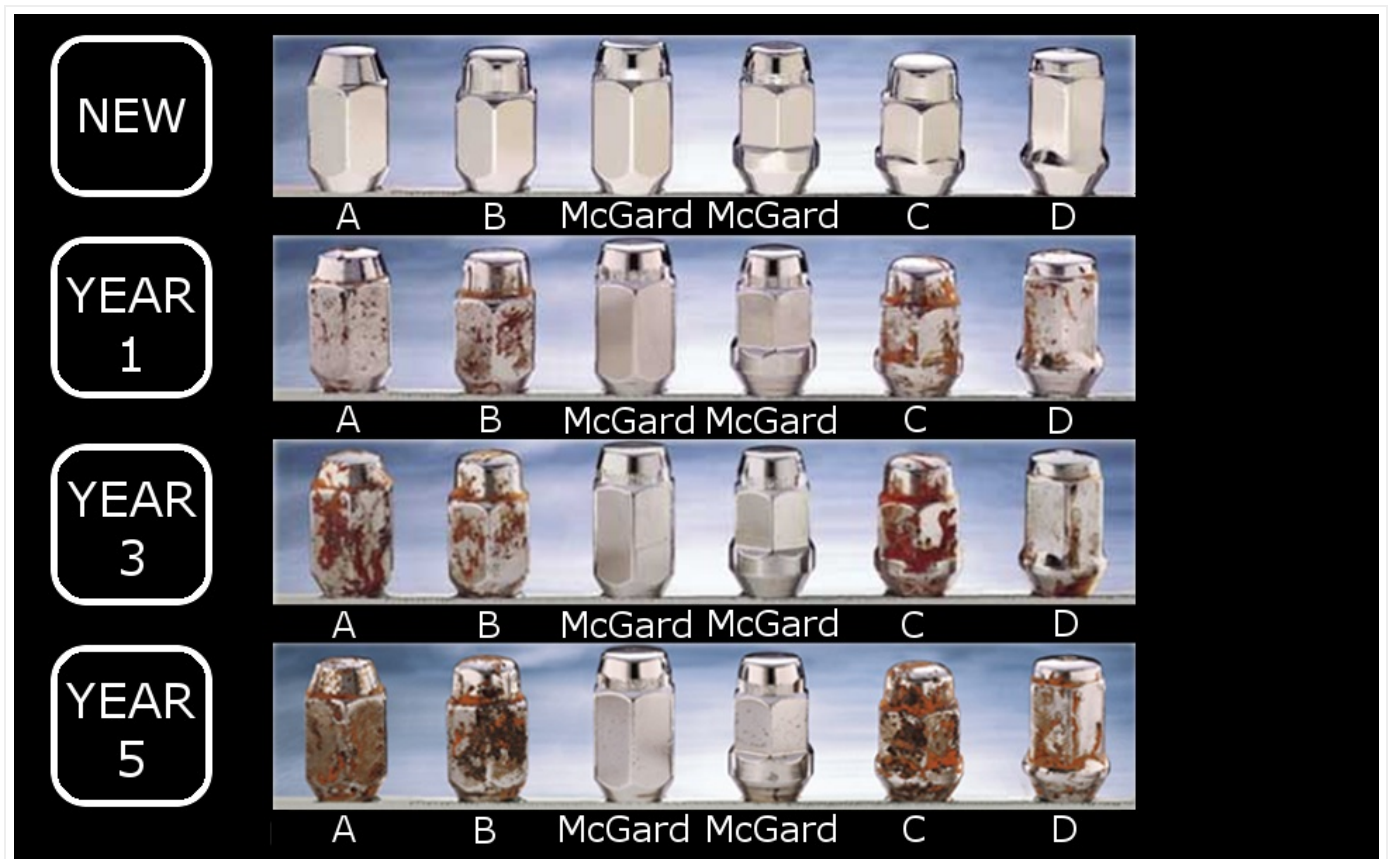
Image: A visual comparison demonstrating the long-term durability of McGard lug nuts (labeled 'McGard') compared to other brands (labeled 'A', 'B', 'C', 'D') over 1, 3, and 5 years, highlighting McGard's resistance to rust and corrosion.
