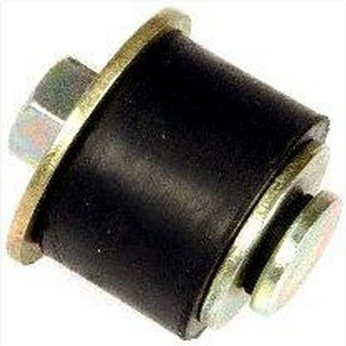
Figure 1: The Dorman 2610 Rubber Expansion Plug. This image shows the black neoprene plug with a metal bolt and washer assembly used for expansion and sealing. The bolt head is visible on one side, and the washer and nut mechanism on the other, which compresses the rubber to create a tight seal.
