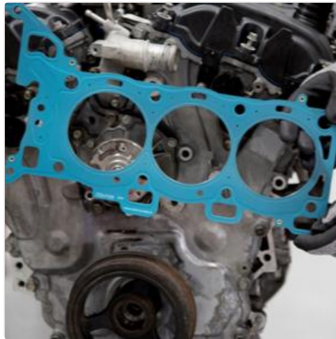
Image 4.1: A head gasket being positioned on an engine block during installation.
