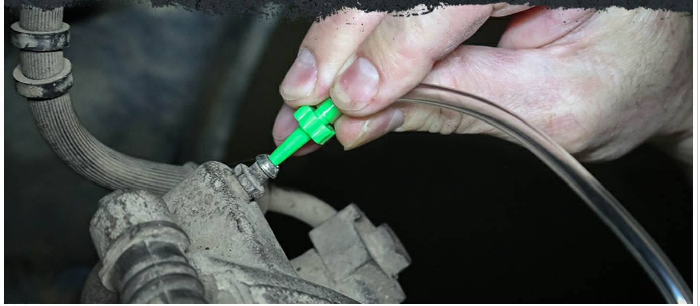
Figure 4.2: Transparent hoses allow for clear observation of fluid and air bubbles during the bleeding process.
