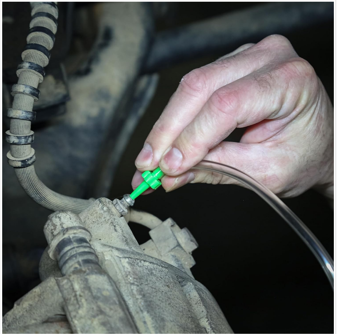
Figure 3.1: Securely attach the tapered fitting to the brake bleeder valve.
