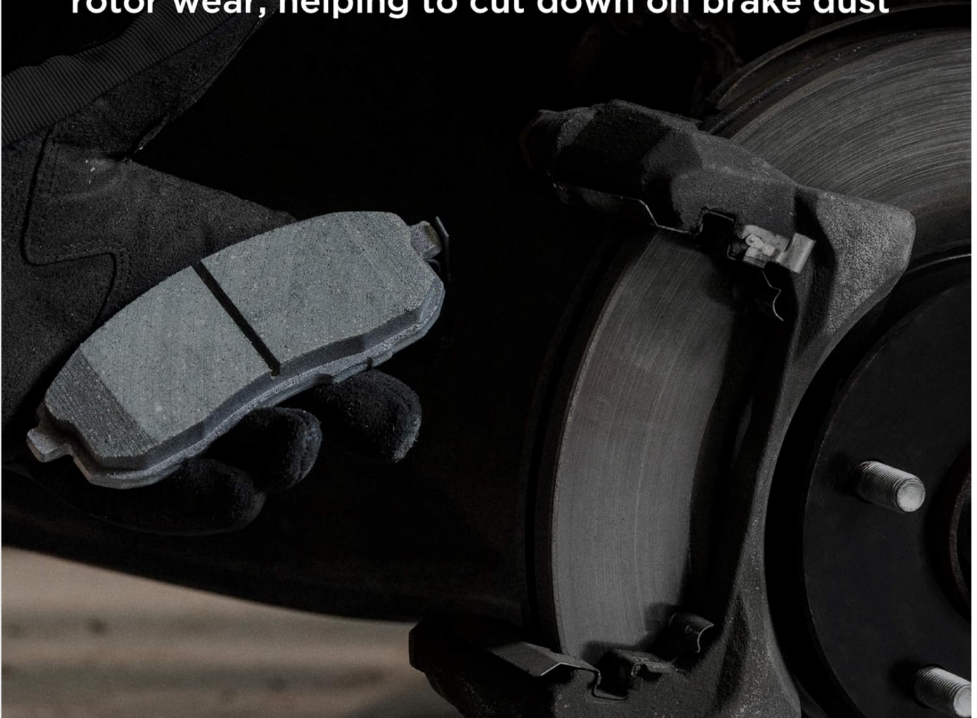
Image: A gloved hand holding a new brake pad, positioned near a vehicle's brake rotor and caliper, illustrating the installation process.
