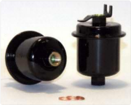
Image 2: Side view of the ProTech 523 Fuel Filter, showing two filters and a washer. One filter is upright, displaying its top connection, while the other is on its side, revealing the internal connection point. A copper washer is also visible, indicating its use in sealing the fuel lines.
