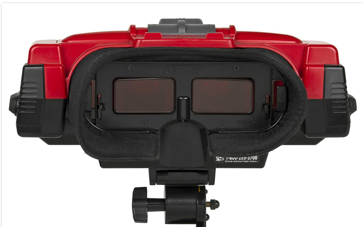
Figure 2: Virtual Boy eyepiece showing focus and IPD adjustment controls.
